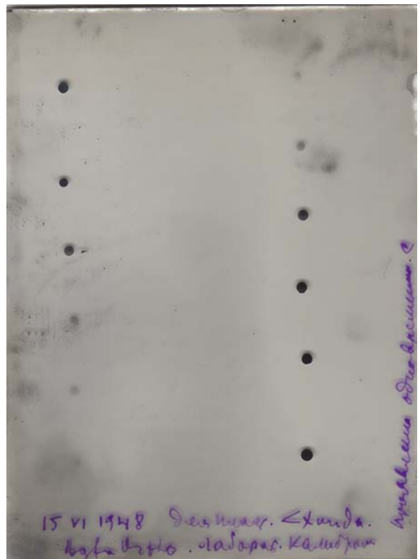
Fig.11. Calibrating images obtained with the tube photometer in laboratory for estimation of emulsion sensibility
